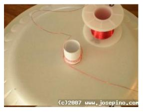
Start making the coil, keep the magnet inside so you don't crush the paper cylinder.
