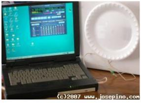
As you can see on the picture, I did use a foam plate. I tried other materials and I found the best quality of the sound is produced by a lightweight material but strong enough to avoid excessive vibration. Paper plates are too soft, plastic disposable plates produces excessive vibration.
