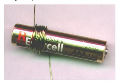
Now carefully pull the coil off of the form, holding the wire so it doesn't spring out of shape.
